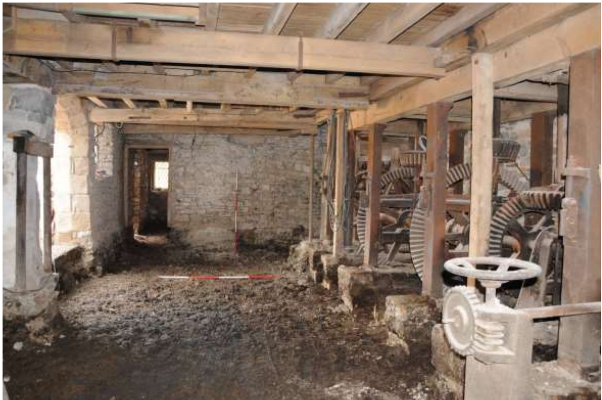
Water-power machinery in situ , during archaeological recording of a mill prior to conversion (© The JESSOP Consultancy [TJC Heritage Ltd])
