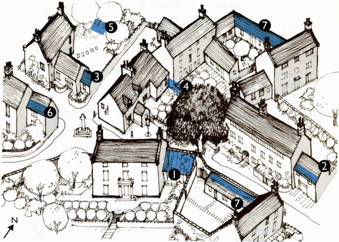
Figure 5 - Illustrative guidance for locating solar technologies in a traditional village scene.
