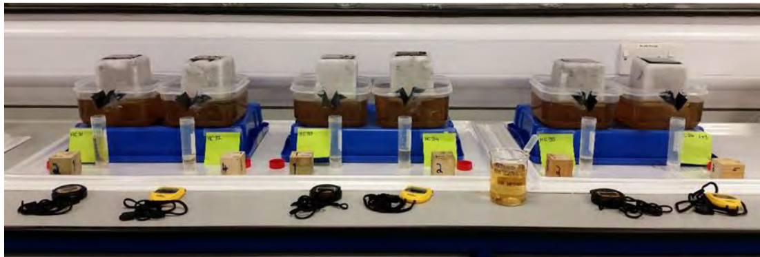
Figure 5.5 Experiment set-up of surface peat samples to measure K using the modified cube method.
