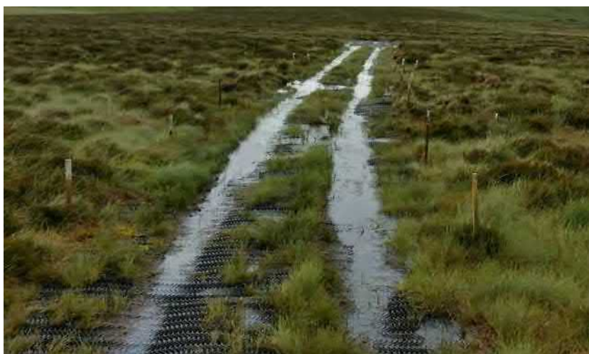
Figure 6.25 Evidence of channelization and redirection of overland flow along track at experiment site.
