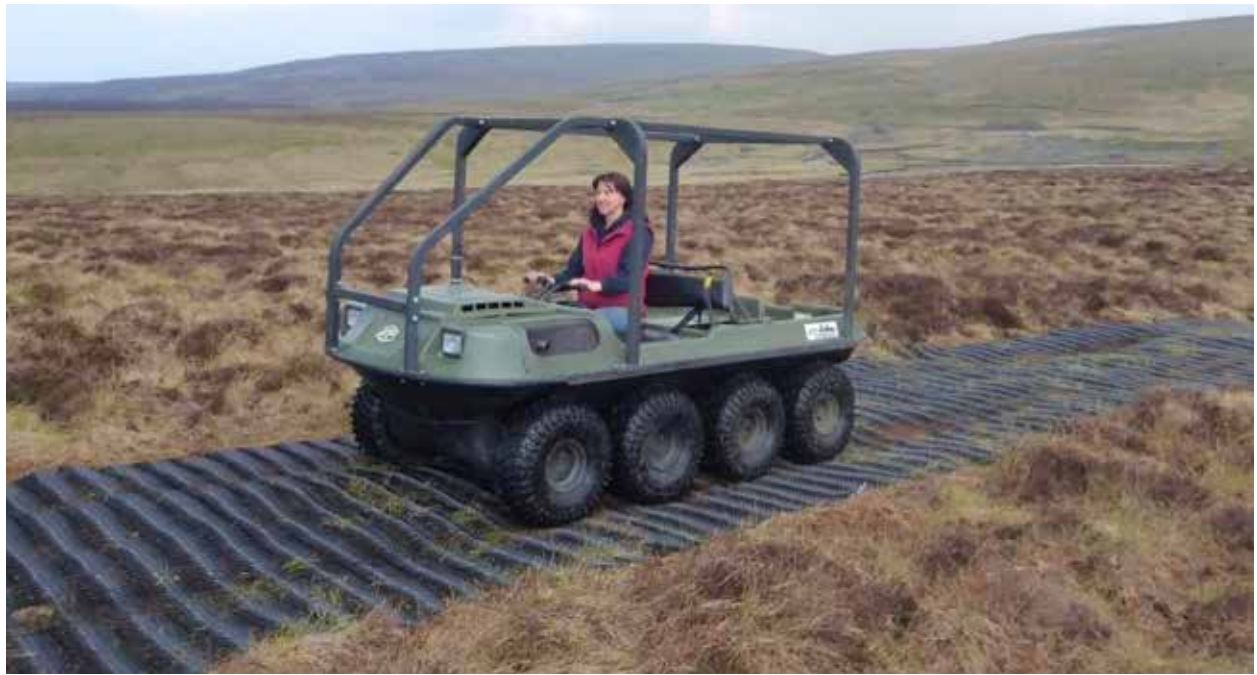
Plastic mesh track trial with the Argocat (but also suitable for quad bikes)
