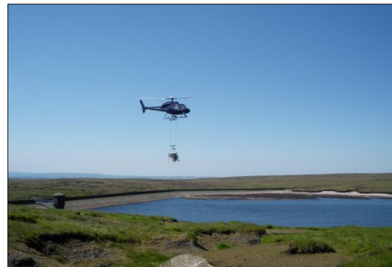
Fig.9 Aerial application of lime using a spinning hopper
