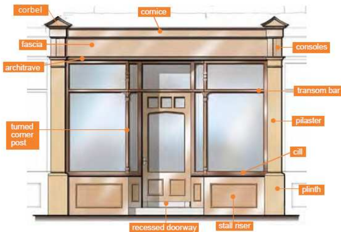
14. Main Components of a Traditional Shop Front
